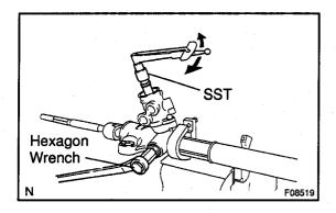
(f) Using SST, a torque wrench and hexagon wrench (19 mm), tighten the rack guide spring cap until the preload is within the specification.
