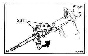
(b) Using SST, hold the steering rack steadily and using another SST, remove the rack end.
