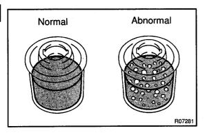
(e) Check for foaming or emulsification. If there is foaming or emulsification, bleed power steering system (See page SR–5).
