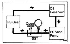
(g) With the engine idling, open the valve fully.
