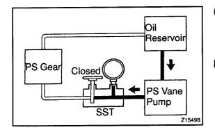
(f) With the engine idling, close the valve of the SST and observe the reading on the SST.
