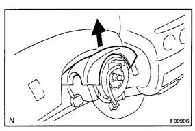
(e) Slide the column upper cover and remove the spiral cable.
