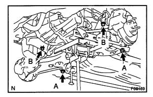
(c) Install the front suspension member with lower suspension arm and PS gear assembly with the 4 bolts.
