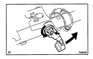
(c) Install the adjusting nut by rotating it counterclockwise in the specified torque so that the locking load (load applied to when a knob is operated) of the tilt lever will be 43 – 91 N (4.4 – 9.3 kgf, 9.7 – 20.5 lbf).
