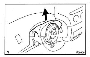
(b) Slide the column upper cover and install the spiral cable.
