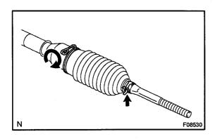
(b) After winding and tightening the clamp around the circumference of the boot twice, twist it several times, and install it.
