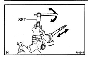
(c) Using SST, turn the control valve shaft right and left 1 or 2 times.
