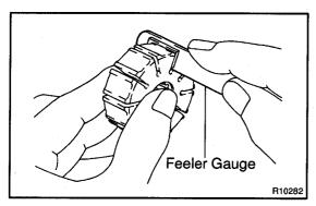
(b) Using a feeler gauge, measure the clearance between the vane pump rotor groove and vane plate.
