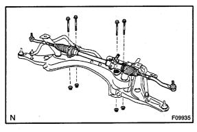
(d) Install the manual steering gear assembly with the 4 bolts and nuts to the front suspension member.
