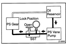
(i) With the engine idling and valve fully opened, turn the steering wheel to full lock position.
