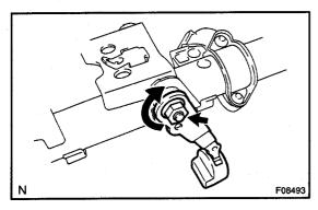
(b) Remove the adjusting nut, tilt lever, stopper, tilt lever lock bolt and break away bracket.
