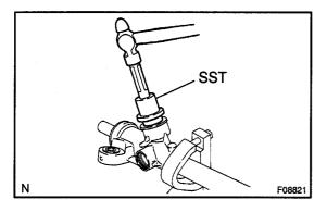
(e) Using SST and a hammer, tap in the oil seal. SST 09517–12010
