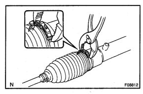
(b) Install the boot, clip and a new clamp.
