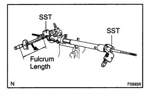
(d) Using SST, hold the RH rack end steadily and using another SST, torque the LH rack end.
