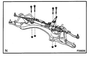
(f) Remove the 4 bolts, nuts and PS gear assembly from the front suspension member.
