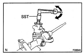
(e) Using SST and a torque wrench, check the preload. SST 09616–00010
