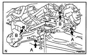
(c) Install the front suspension member with lower suspension arm and manual steering gear assembly with the 4 bolts.
