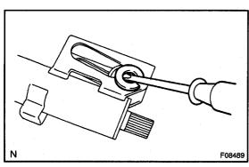
(b) Using a screwdriver, remove the 2 No. 1 support collars.
