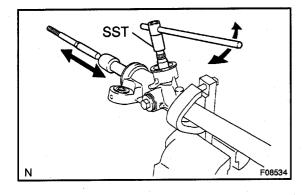
(e) Using SST and a torque wrench, tighten the rack guide spring cap until the preload is within specification.
