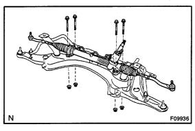
(d) Install the PS gear assembly with the 4 bolts and nuts to the front suspension member.
