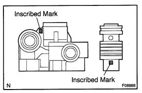
If necessary, replace the flow control valve with the one having the same letter as inscribed on the front housing.
