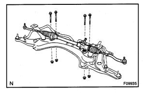
(c) Remove the 4 bolts, nuts and manual steering gear assembly from the front suspension member.
