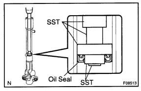
(b) Install the oil seal to SST, and press them into the rack housing.
