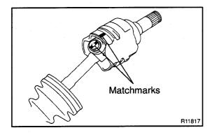
(c) Place matchmarks on the inboard joint shaft and tripod. **NOTICE:**
