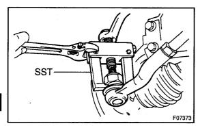
(b) Using SST, disconnect the tie rod end. SST 09628–62011
