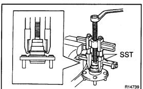
(b) Using SST, remove the inner race (outside) from the axle hub.
