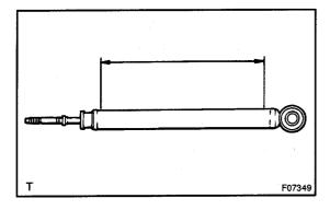
2. DRILL HOLE TO DISCHARGE GAS FROM CYLINDER Using a drill, make a hole in the cylinder as shown in the illustration to discharge the gas inside.
