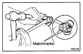
(b) Place matchmarks on the outboard joint shaft and tripod. **NOTICE:**
