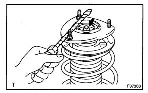
(f) Using 2 nuts and a screwdriver or an equivalent to hold, install a new center nut.
