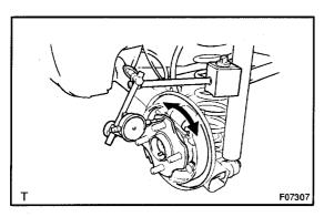
(b) Using a dial indicator, check the deviation at the surface of the axle hub outside the hub bolt.
