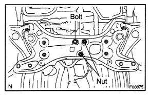
(b) Install the 2 No. 1 engine hangers with the bolts in the correct direction.
