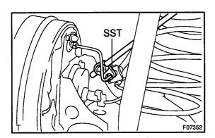
(b) Using SST, connect the brake line to the flexible hose. SST 09023-00100
