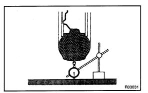
(b) Using a dial indicator, check the tire runout.
