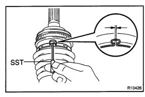
(g) Using SST, adjust the clearance of the large clamp. SST 09240-00020
