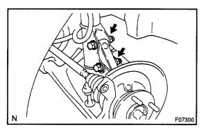
7. REMOVE STEERING KNUCKLE WITH AXLE HUB
