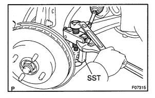
(b) Using SST, disconnect the tie rod end from the steering knuckle.
