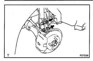
(b) Remove the 2 nuts on the lower side of the shock absorber.
