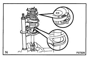
(b) Install the coil spring to the shock absorber.
