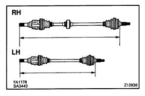
(b) Make sure that the 2 boots are not stretched or contracted when the drive shaft is at standard length.
