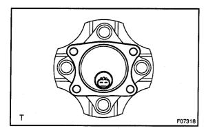
(b) Place the ABS speed sensor on the axle hub so that the connector is set at the bottom under the on-vehicle condition.
