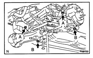
(c) Install the suspension member with the 4 bolts.
