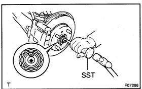
(c) Using a dial indicator, check the backlash near the center of the axle hub.
