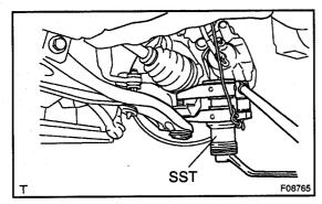
(b) Using SST, disconnect the lower suspension arm from the steering knuckle.
