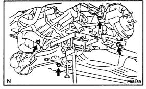
(b) Remove the 4 bolts and lower the suspension member.
