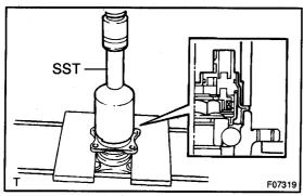
(c) Using SST and a press, install a new ABS speed sensor to the axle hub.
